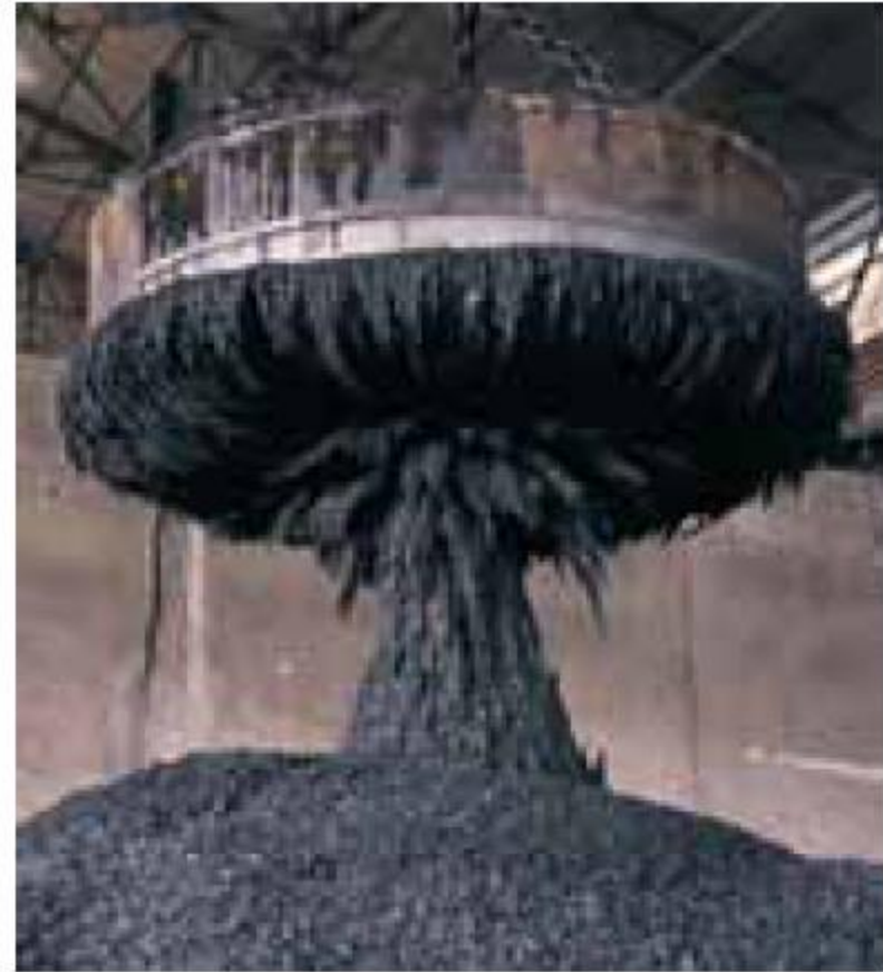
Fig. 28-1 Using an electromagnet to collect and transport scrap metal at a steel mill. (Digital Vision/Getty Images)
